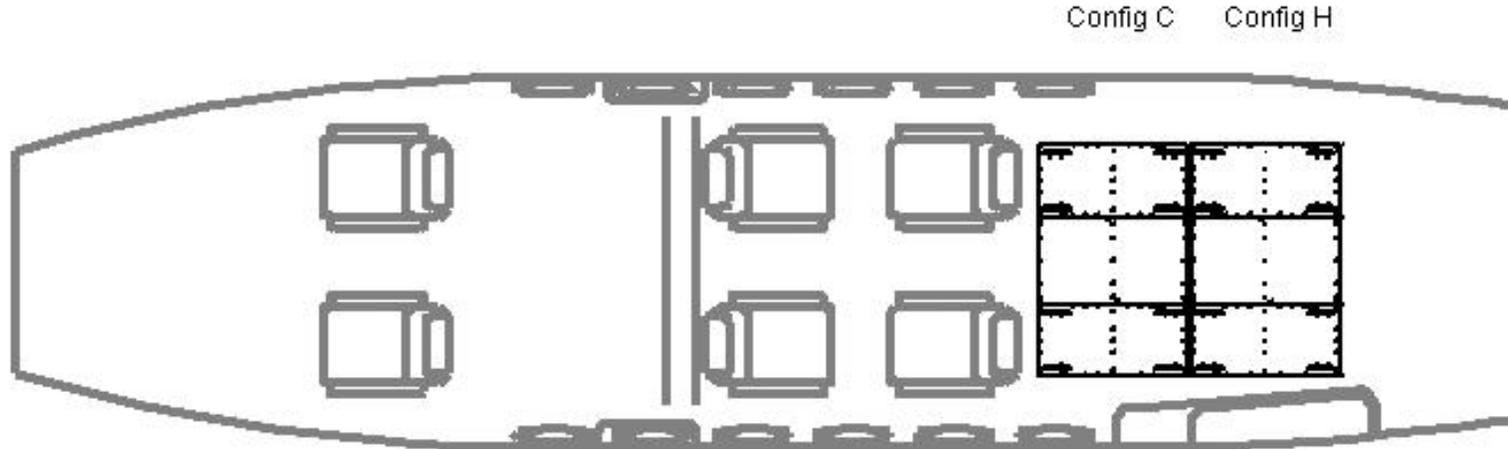
Aerospace Resources C-12 (King Air 350) **Configuration C** has a weight capacity of 400 pounds of freight and is 30.0 inches by 46.8 inches. The three decks used for Config C are contained in **Kit K003** (see Kits, Assemblies and Parts). Recommended for use with **Cargo Net Assembly FA00 003**. Also, **Restraint Bar FA00 005** may be used at operator's discretion to keep cargo from shifting longitudinally under the Cargo Net Assembly.
