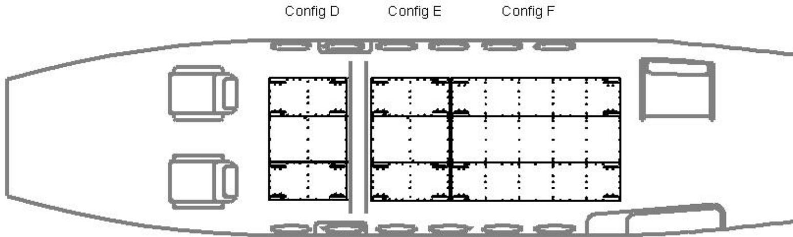
Aerospace Resources C-12 (King Air 350) **Configuration D** has a weight capacity of 400 pounds of freight and is 30.0 inches by 46.8 inches. The three decks used for Config D are contained in **Kit K003** (see Kits, Assemblies and Parts). Recommended for use with **Cargo Net Assembly FA00 003**. Also, **Restraint Bar FA00 005** may be used at operator's discretion to keep cargo from shifting longitudinally under the Cargo Net Assembly.
