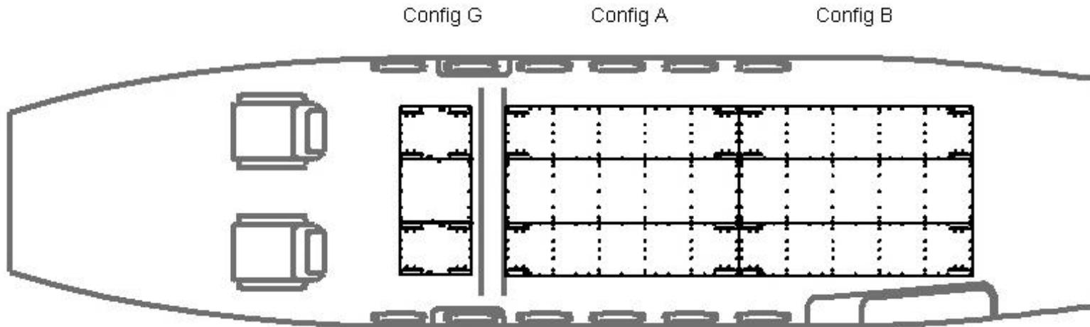
Aerospace Resources C-12 (King Air 350) **Configuration G** has a weight capacity of 300 pounds of freight and is 20.0 inches by 46.8 inches. The three decks used for Config G are contained in **Kit K004** (see Kits, Assemblies and Parts). Recommended for use with **Cargo Net Assembly FA00 003**.
